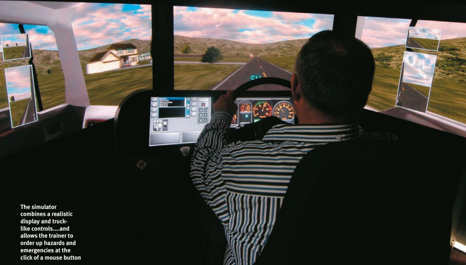
The simulator combines a realistic display and truck-like controls...and allows the trainer to order up hazards and emergencies at the click of a mouse button
