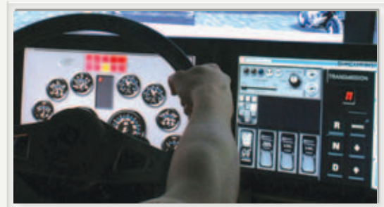
Glass dash offers flexible gauge placement similar to common fire truck and ambulance models.
