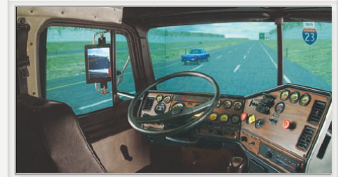
Fully operational cab, with real working instrument panel, gauges and controls
